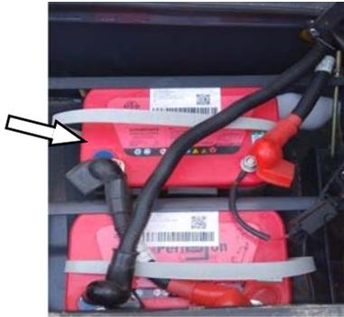
2. Measure the battery voltage through battery tester and multimeter.
