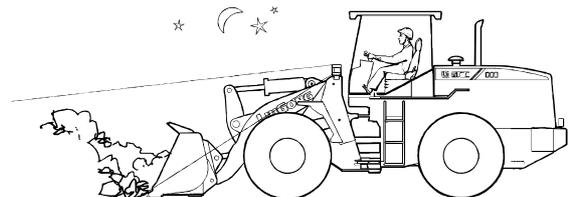
If driving or operating the machine with a bad view or in a crowded area, you should work with a signalman, keep the signalman within the field of your vision, and coordinate your hand signal.
