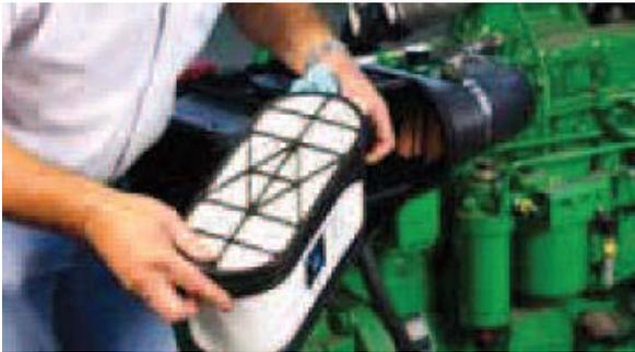
4. Take out the safety filter element. Use the handles on the safety filter element to pull it towards the filter housing center, and then take it out.
