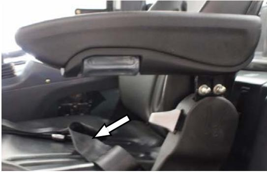
Adjust length of the seat belt before use in order to ensure safety and comfortability. Length of the seat belt can be adjusted by moving position of catch on the safety belt.
