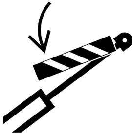
For those parts fitted with shields, if it is necessary to remove shields in order to perform maintenance, always install the shields after the maintenance is performed.
