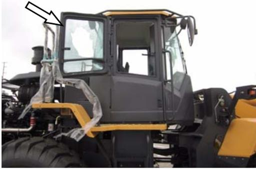
Pull the latch unlocking handle to unlock the window, and then pull the inner handrail backward to close the right window.
