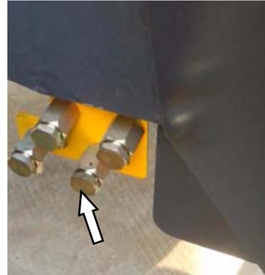
4. Tighten the oil drain plug.
