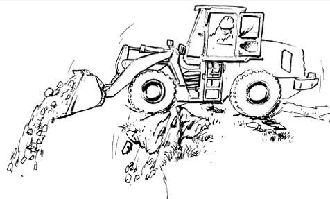
When driving the machine on a slope, make it straight up and down and neither make turn on the slope nor drive it transversely on the slope to prevent tipping. The distance between bucket and ground should be 200-300mm (7-12in).
