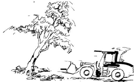
Consider filled or unstable ground. Be certain the condition of the work site is stable and capable of supporting the machine during operation. Do not operate the machine close to an unstable drop off. Operation of the machine on shoulders, drop off's, or filled areas could cause the machine to become unstable, presenting a work hazard.
