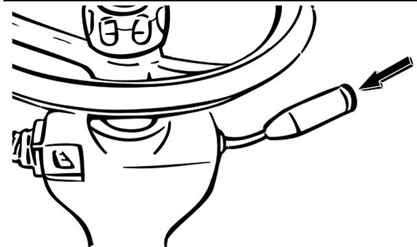
The horn will sound by pressing the horn button at the end of combination switch.
