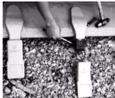
5. Install new tip on the tooth. Drive the pin into the snap ring, tooth, and tip from the side of the snap ring.
