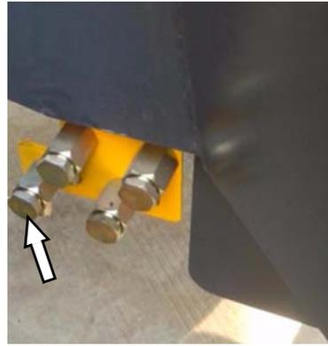
8. After draining out coolant, close the water drain plug.
