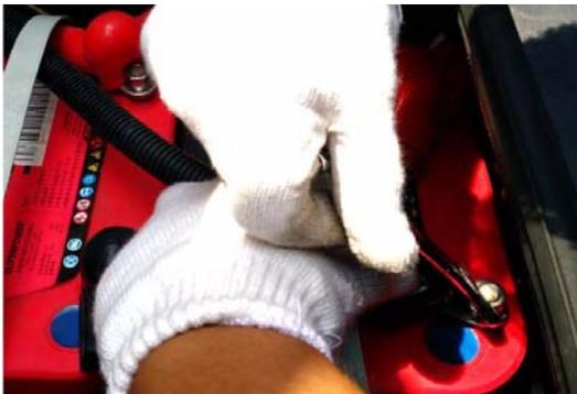
4. Connect the cables after finishing charging. Connect the positive cable first.
