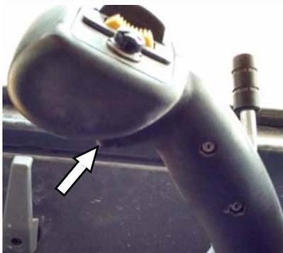
See above picture shows, the arrow direction is the operation direction of the KD key.
