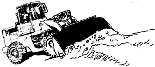
4. When the bucket is loaded, tilt it back against the stops. Carry the loaded bucket approximately 40 cm (15 inches) above the ground when moving to the dump area.
