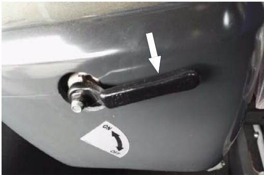
Turn the pilot shutoff lever to horizontal (ON) position, the work implement will move when operating the control lever; turn the pilot shutoff lever to vertical (OFF) position, the work implement will not move when operating the control lever. This can prevent the accident caused by misoperation.
