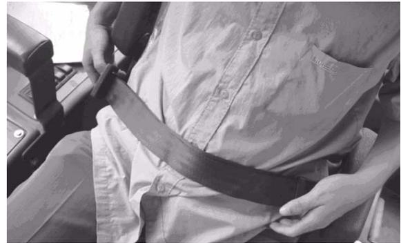
A red button is provided by side of the buckle. Press the button, the catch will spring up from the buckle.
