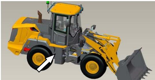
1. Unscrew the breather filter oil filler cap of the hydraulic oil tank slowly to release the pressure. Take off the oil filler cap.
