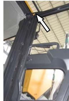
After the left door is opened to a particular opening, it can be opened completely and positioned automatically by an air spring, which is located on the top of the left door. Pull the inner handrail backward to close the left door.
