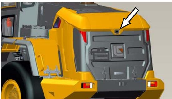
The camera will work after the monitor system is powered on. Ensure the operator has a good visibility during operation. The rear view mirror and moonitoring system can help the driver with getting a good view of the rear side.
