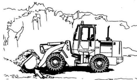
2. Apply down pressure to the bucket as the loader starts forward. Return the lift control to HOLD when sufficient penetration is obtained.
